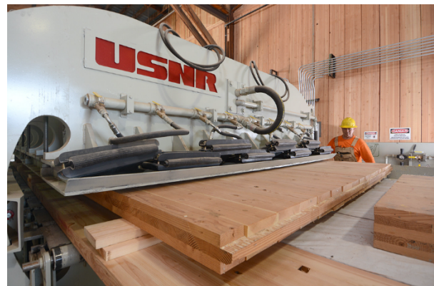
Figure 12: CLT press. An understanding of a manufacturer's production capabilities informs an efficient grid design. Source: DR Johnson
