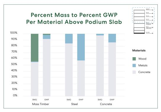
Figure 9. Relative contribution of materials to mass and to GWP of each system, above the podium slab.
