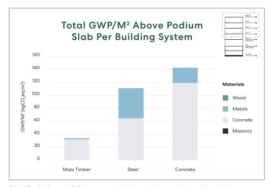
Figure 8. Total framing system GWP per square meter of each system with representative material contribution.
