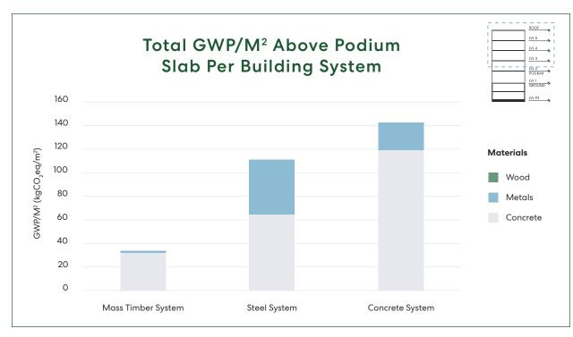
Figure 1. Total GWP per square meter above the podium slab for three building systems, showing contributions in each from three material categories. Mass timber's GWP contribution of 0.33 per m2 is so small, it does not appear in the chart.
