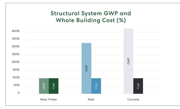
Figure 15. Comparison of the structural system GWP above the level two podium slab and the whole building cost of the three systems.
