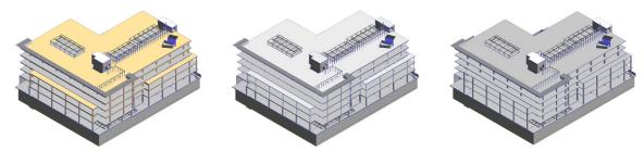
Figure 4. Isometric representation of the three structural framing systems: mass timber, steel, and concrete.
