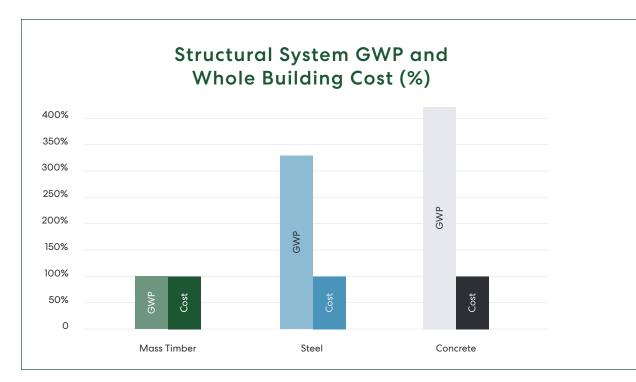
Figure 2. Comparison of the structural system GWP (above the level two podium slab) and the whole building cost of the three systems.
