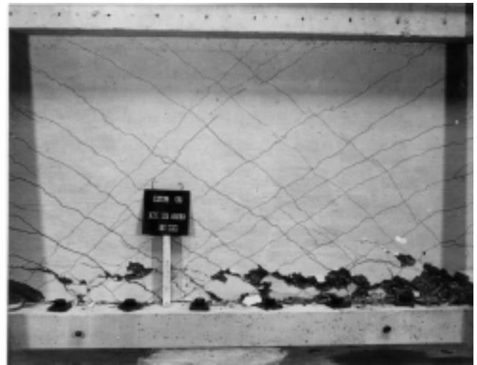
Splitting and Crushing of Concrete at Base of Wall
